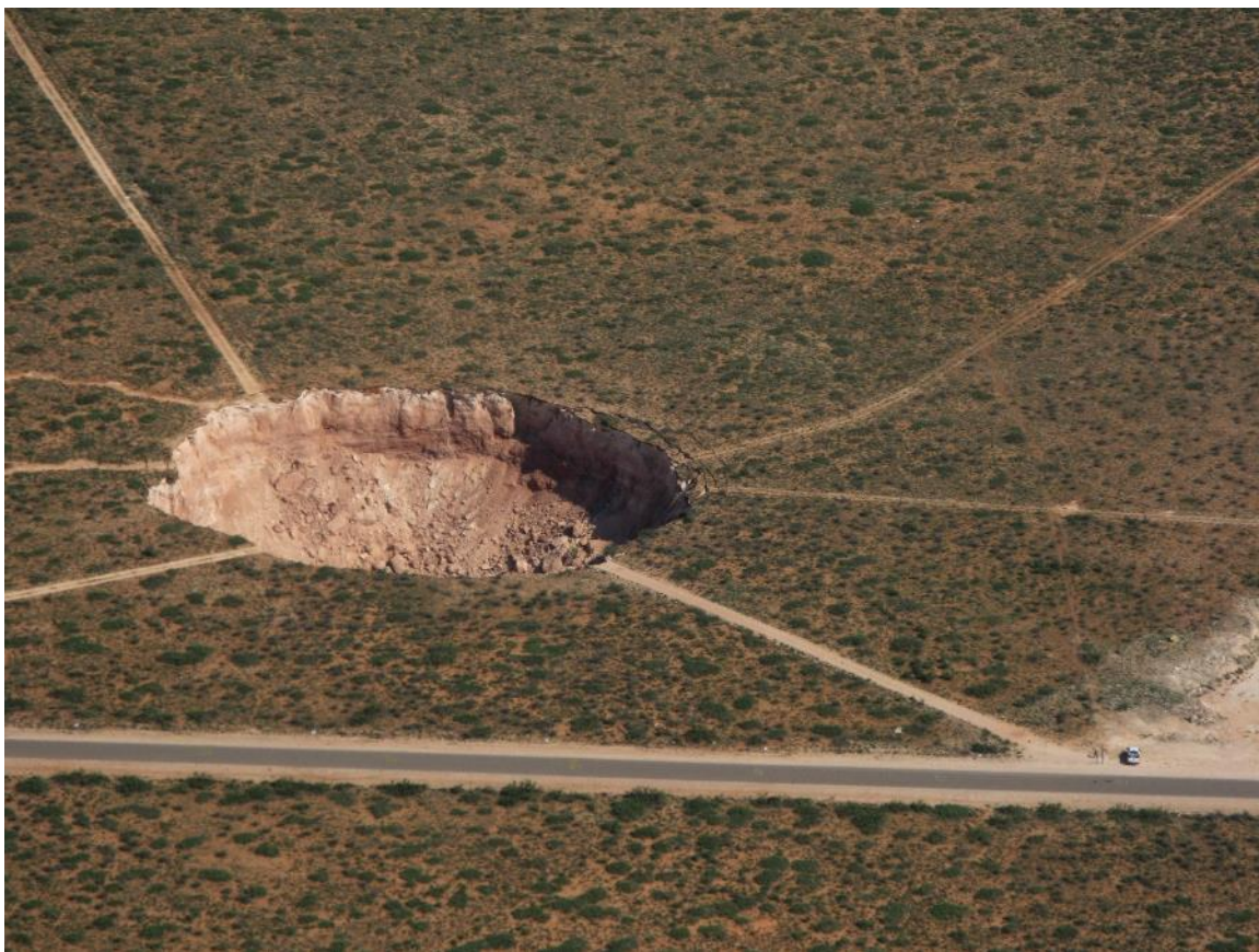
Figure 6-129 JWS sinkhole in northern Eddy County, about three weeks after initial brine well collapse. Pickup truck in lower right corner for scale.
